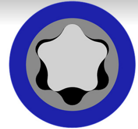
RECOMMENDED ROTOR / STATOR FIT
