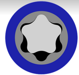
RECOMMENDED ROTOR / STATOR FIT
